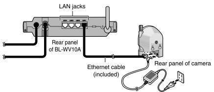
Cameras must be connected and configured by Quick Setup one at a time.
