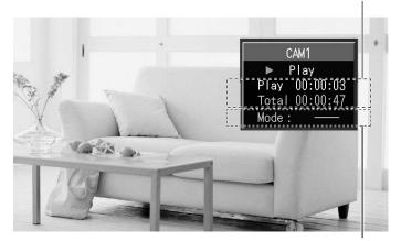
The recording mode (HIGH, LOW, LONG, or —) will be displayed. Movies recorded manually while monitoring the camera image will be recorded at the monitoring resolution and displayed as — .
